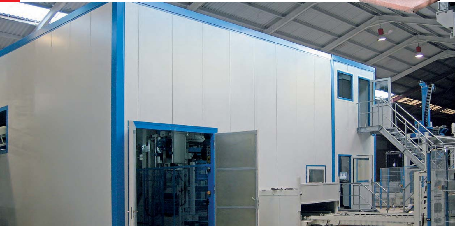
Machine coverage with connected control- and switch cabinet cabin for new installations and retrofitting.
