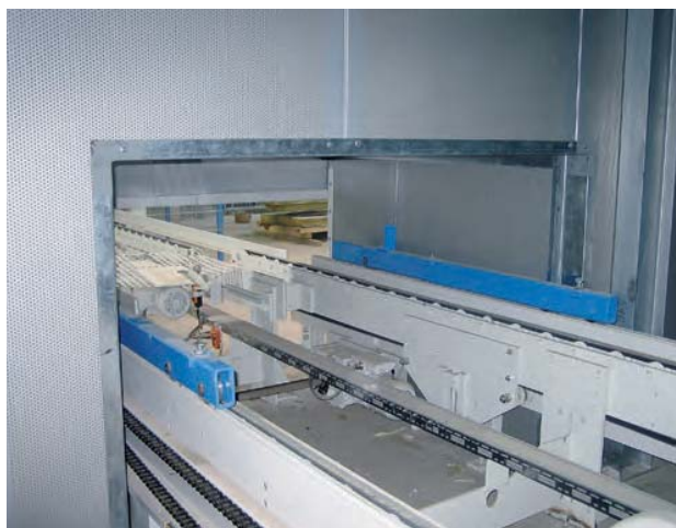
Sound protection tunnel for pallet feed and further transportation. For different block heights with height-adjustable sliding element.
